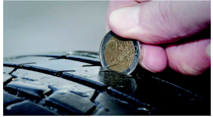
The two-euro coin test: if the 4-mm silver-colour rim of the coin is visible above the tread pattern of the tyre, it is advisable to consider replacing the tyre or taking special care in the rain.
